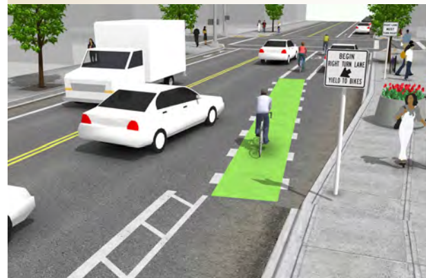
Colored Pavement Treatments
