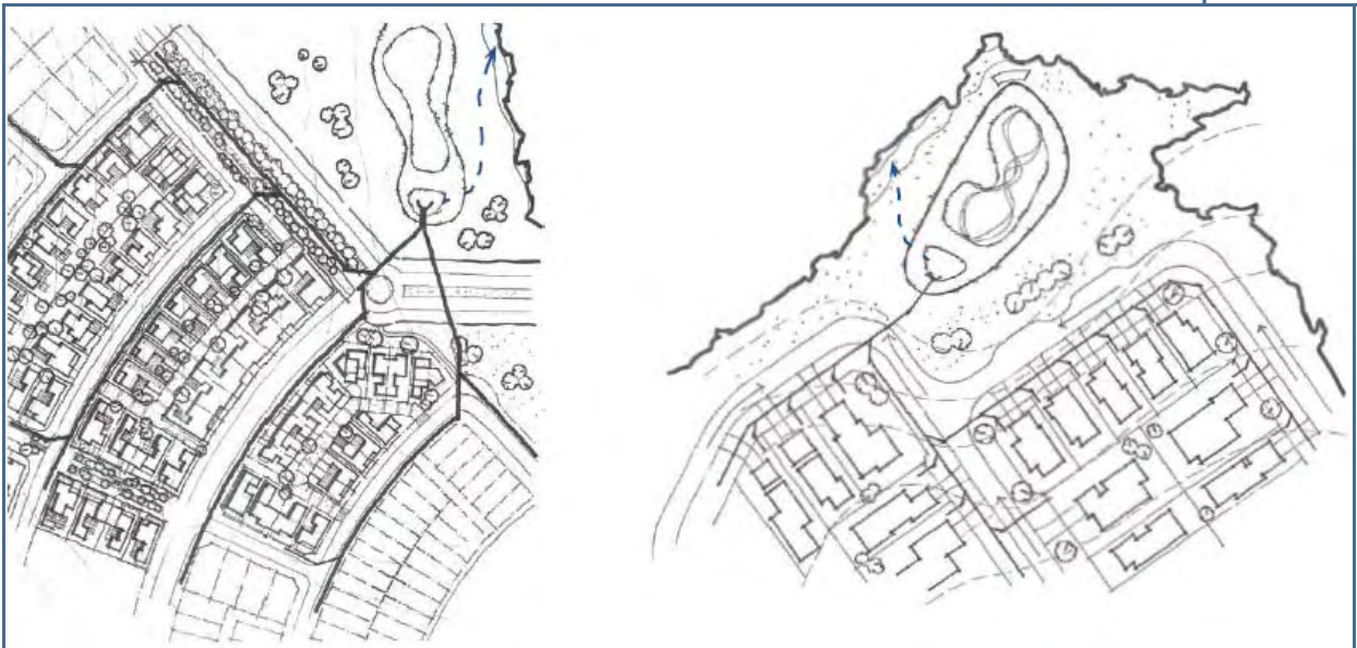
End-of-pipe wetland may be appropriate if suitable open space is available.
