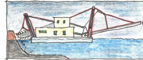
GOLD MINING BARGE, NOTE ANGLED TOWERS AND FORKED CABLE SUPPORTS
