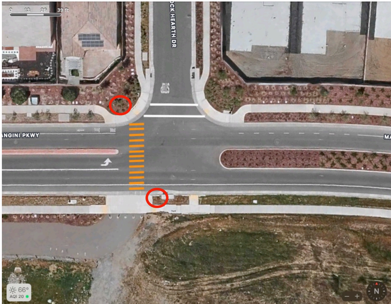
Proposed pedestrian crosswalk at Mangini Pkwy and Rock Hearth Dr (The red circles indicating pedestrian-controlled crosswalk lights)
