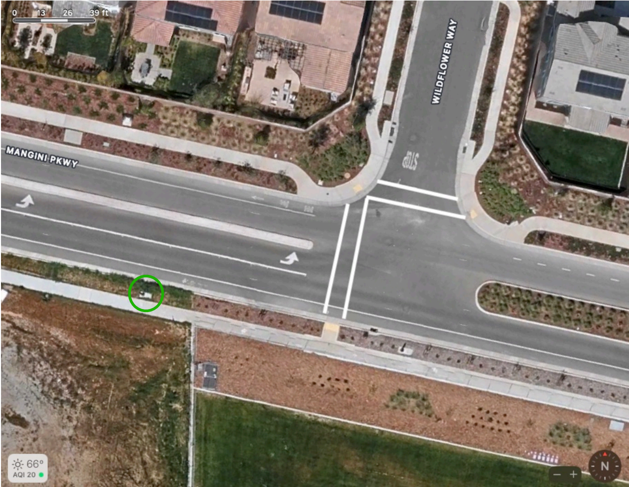
Proposed pedestrian crosswalk at Mangini Pkwy and Wildflower Way (The green circle indicating existing school zone warning lights)
