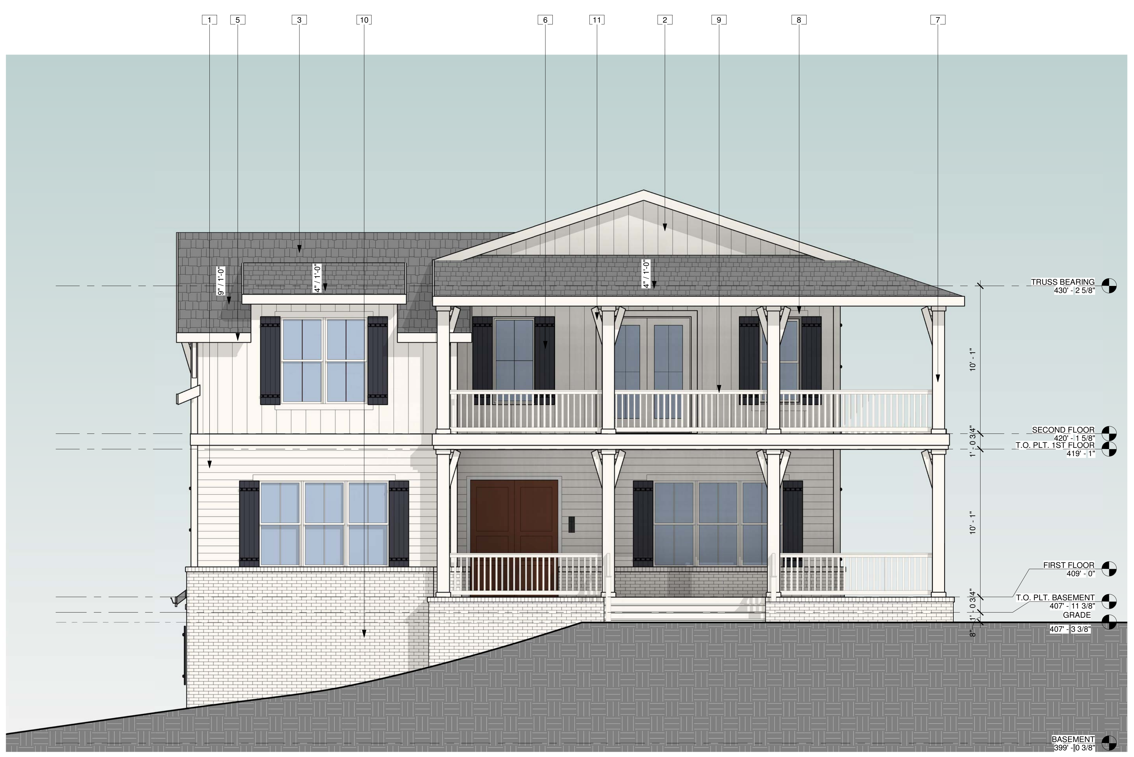
2 FRONT ELEVATION - MAIN BUILDING SCALE: 1/4" = 1'-0"
