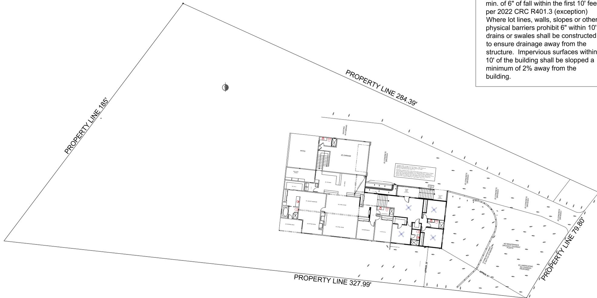
Note: Where applicable, embed all utility lines with a minimum 18" min. coverage (anywhere beyond the foundation)
