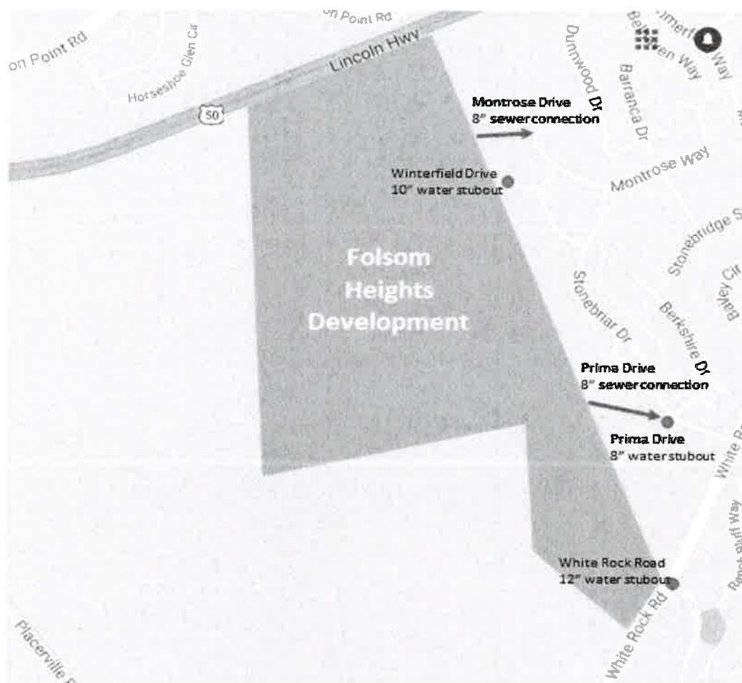
Figure 1-2: Available Tie-In Locations to Existing EID services
